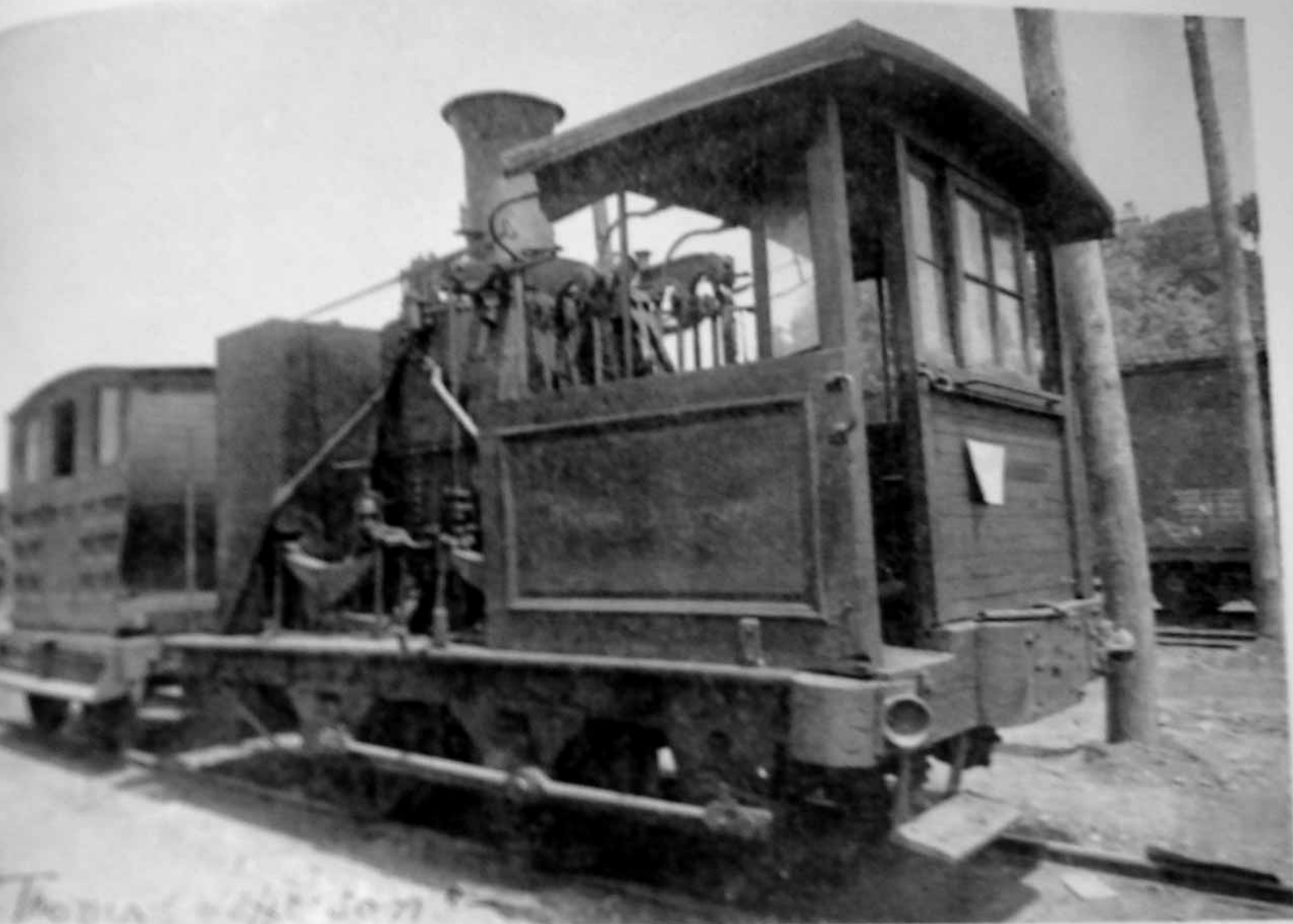
This is a picture of an old engine and passenger car taken about 1900 in the yards of the Ohio Central Railway, now the New York Central, in Charleston. This type of engine had been in use before the Civil War, possibly about 1840, and was apparently being stored in the Charleston yard. The Savage home on Capitol Hill can be seen in the back ground.
